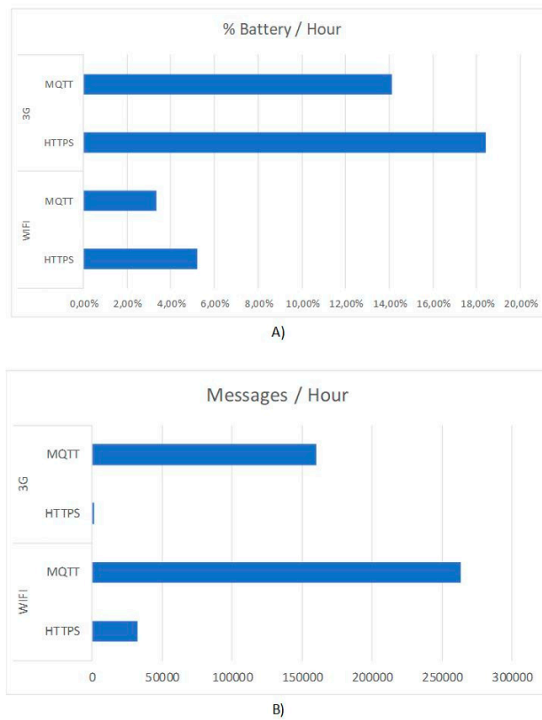
Figure 2. (A) Battery percentage consumed per hour and (B) messages sent per hour (results grouped by protocols and networking technologies).
