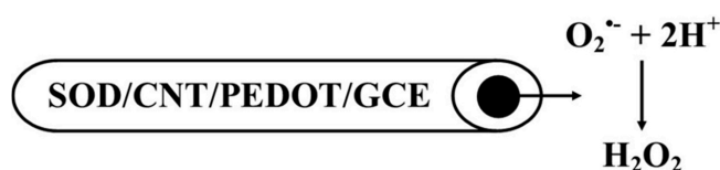
Figure 5. Schematic presentation of SOD biosensors based on PEDOT and CNT.
