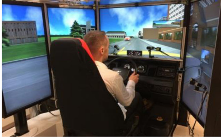
Figure 1. Driving simulator with 6-camera head and eye tracking system
