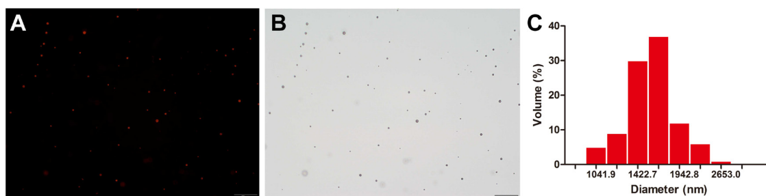
Figure 1: Physical property of MBs. (A) Fluorescence image. (B) Bright field image of MBs. (C) Size distribution of MBs measured by a dynamic light-scattering system. Scale bar = 20 \mu m.
