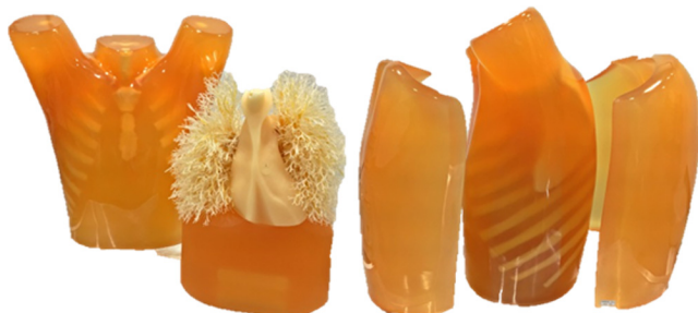
Fig. 1 Anthropomorphic physical phantom Lungman.
