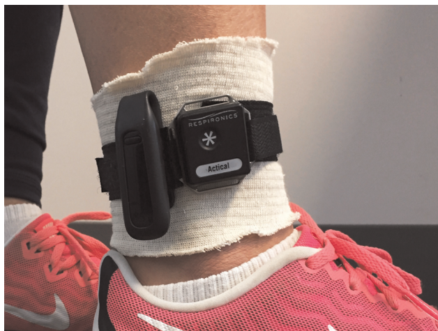
Figure 1 Placement of the Fitbit and Actical devices on the non-paretic ankle using a nylon strap.
