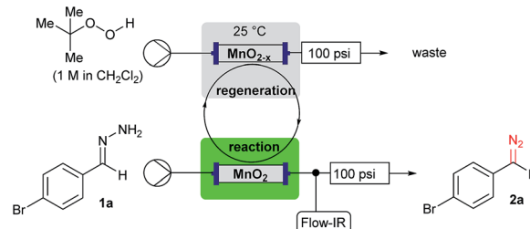
Scheme 7 Flow regeneration of MnO 2 reagent using TBHP.
