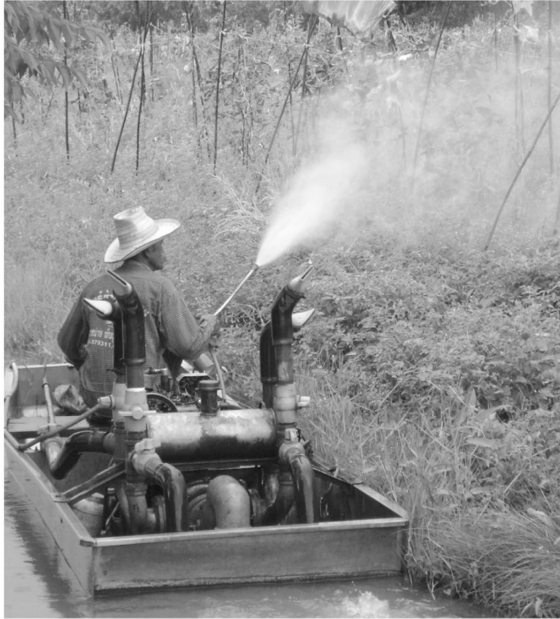
Figure 4. Boat pesticide sprayer (liquid insecticide sits in bottom of open boat).
