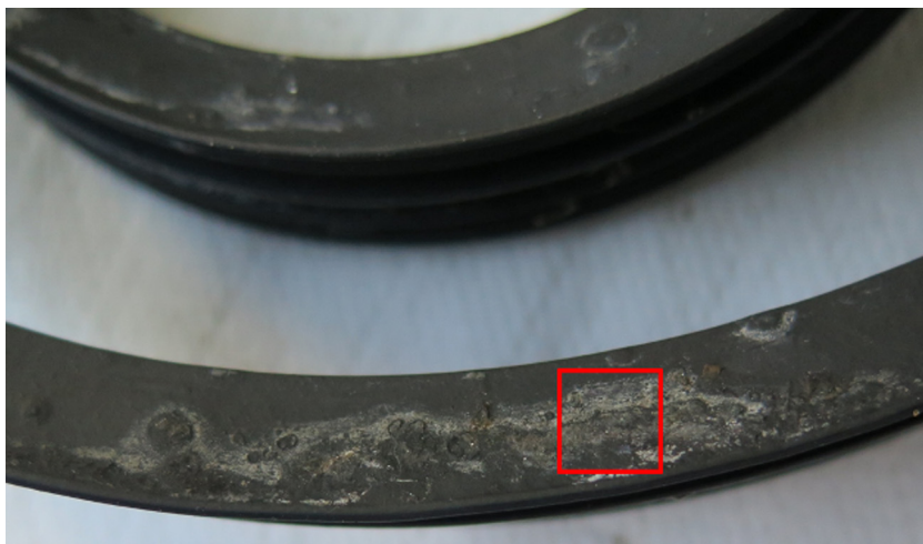
FIG 1 Biofilm formed on rubber seals in residential DWs. Microbial biofilm formation on DW rubber seal; the square (in red) represents the 1-cm 2 sampling site. Biofilm samples from 1 cm 2 were collected by scraping the surface of rubber seal with a sterile scalpel for DNA extraction and further analysis. Sampling was done in situ , with the seal at its original place.
