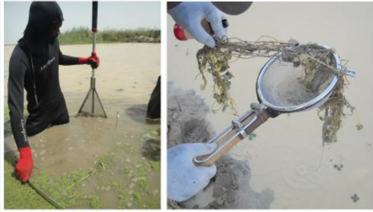
Figure 1. Two different snail scoops designed and deployed to sample snails in schistosomiasis transmission sites in Senegal. Image courtesy of The Upstream Alliance ( http://www.theupstreamalliance.org ), under the terms of the Creative Commons Attribution License CC BY 2.0.
