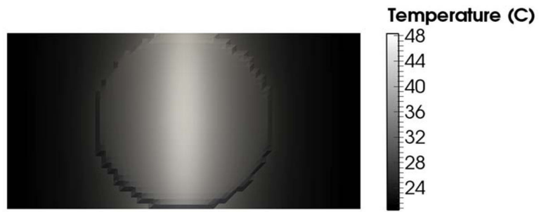
FIGURE 10. SURFACE TEMPERATURE PREDICTION FOR THE HEAT TRANSFER MODEL FOR MOUSE TISSUE AFTER 4 MINUTES OF LASER DURATION.
