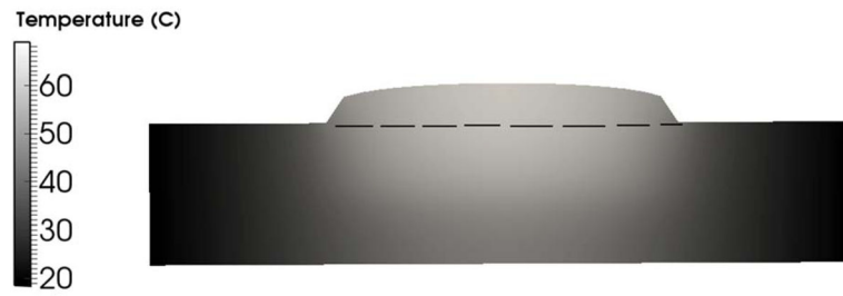
FIGURE 6. PROFILE VIEW OF THE TEMPERATURE GRADIENT THROUGH THE X-Z PLANE. THE DASHED LINE (–) REPRESENTS THE PATCH-TISSUE INTERFACE, WITH THE AREA ABOVE ENCOMPASSING THE PATCH AND THE AREA BELOW ENCOMPASSING THE TISSUE.
