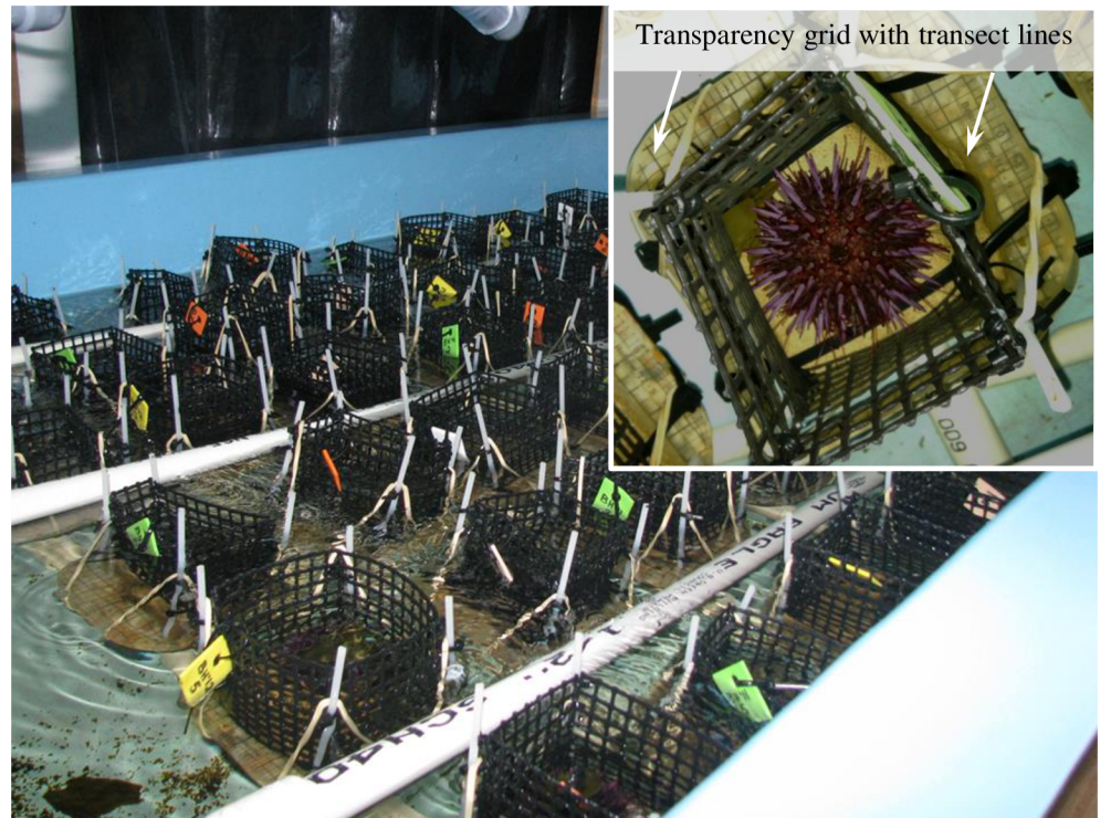
Fig 2. Oblique view of the sea table and experimental layout. Each experimental unit was secured to a PVC-grid on the bottom of the table (not visible, covered by units); the 3 pipes of the sprinkler-system that delivered filtered seawater are visible. For each replicate, the plastic cages surrounding the rocks were secured to the epoxy units with cable ties and plastic posts. The cages restricted urchin movement to the rock surfaces. An overhead view of a single replicate (inset) shows an urchin on one of the sandstone (fine-grain) surfaces and the standardized grid lines for the perpendicular transects used to quantify surface topography. We used a carpenter's contour gauge along these transects to measure the height of the rock (every 0.5 cm) above the epoxy base. These topographic data were used to generate three-dimensional surface plots and calculate rugosity at the start and conclusion of the experiment.
