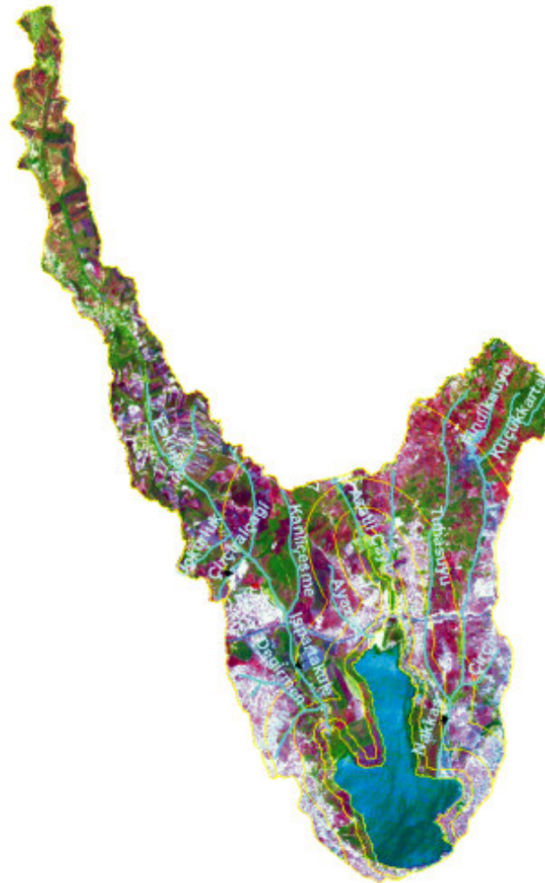
FIGURE 2. A Landsat-5 TM + SPOT-Pan color composite satellite image of Küçükçekmece Water Basin dated 1992. Streams and protection zones were overlaid as vector data, applying GIS software.
