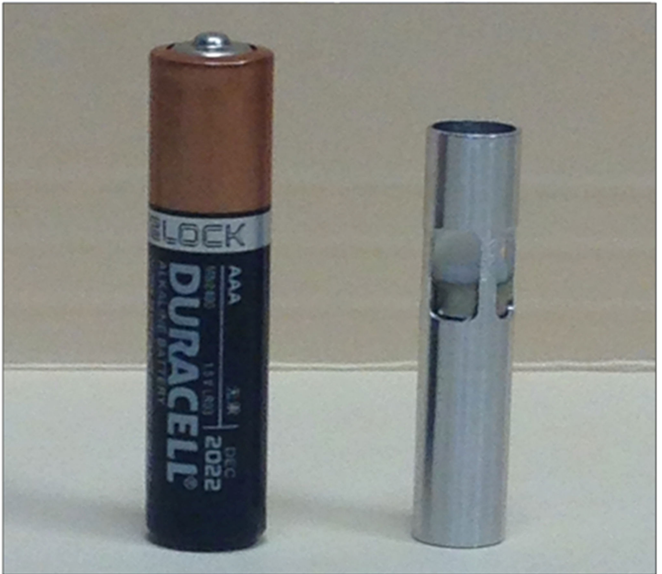
Figure 4. Computer numerical control (CNC)-machined version of Prototype 3 in size smaller than AAA battery. Aluminum casting was used for initial development.
