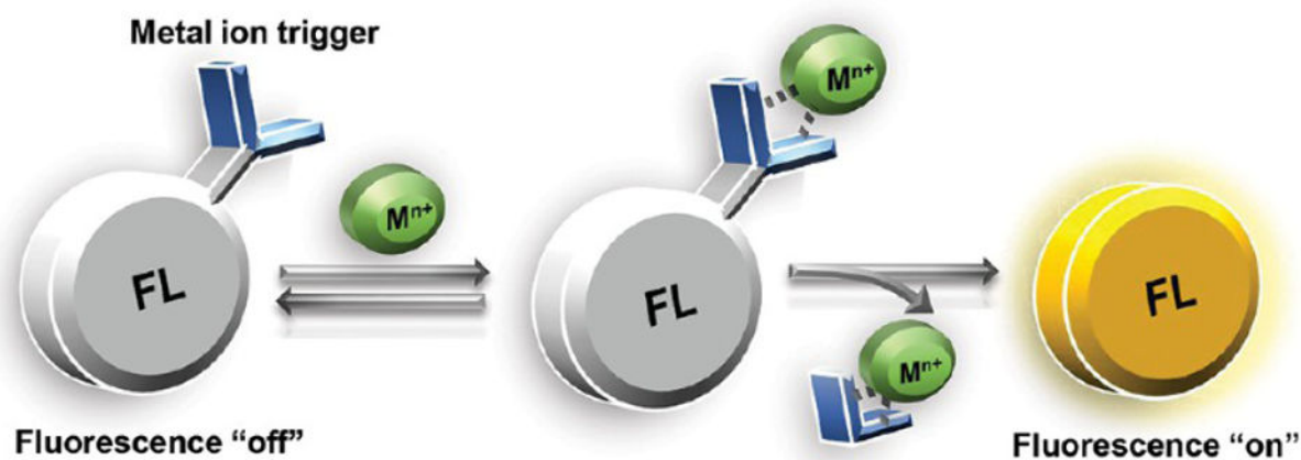
Figure 4. Illustration of recognition-based and reaction-based fluorescent sensors for metal ions. (A) Recognition-based turn-on sensors fluoresce when the metal is bound; they are reversible, turning off when the metal is released. (B) Reaction-based indicators fluoresce after a metal-catalyzed, irreversible chemical event. The fluorophore does not remain associated with the metal after the reaction takes place.
