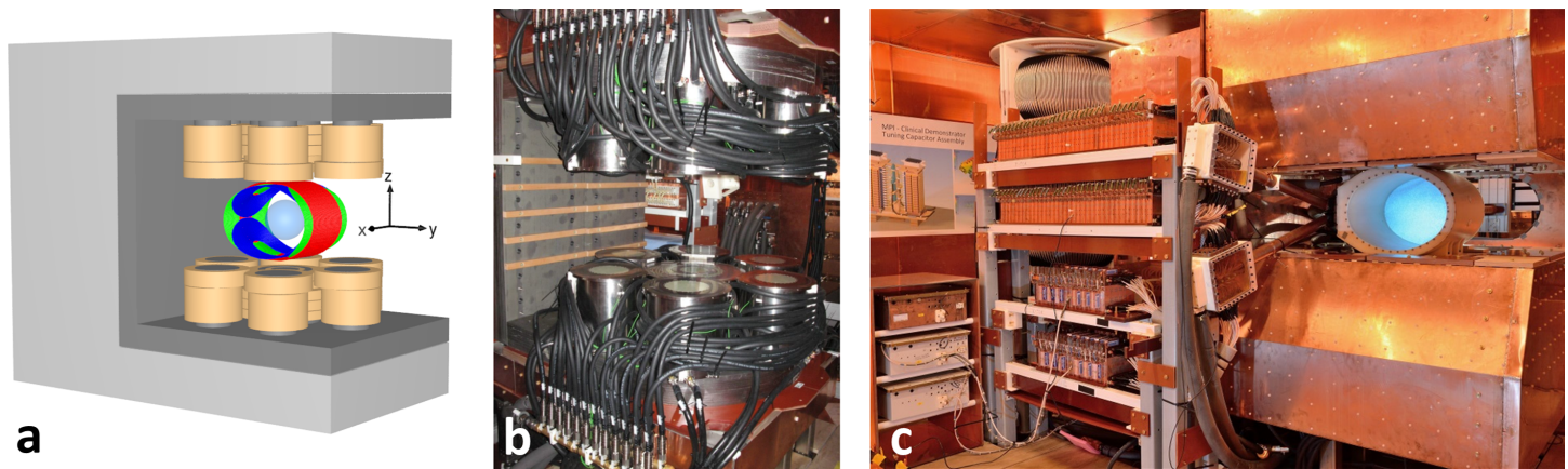
Fig 1. Clinical scale field applicator. (a) Schematic drawing of stacked coils (copper color), iron core (dark gray), and steel yoke (light gray) for low-frequency field generation (< 100 Hz) and flux guidance. A total of 18 coil stacks can be addressed individually by 18 amplifiers. Both at the top and bottom, six outer stacks, a cylindrical stack consisting of two segments, and a central inner stack are mounted. The elliptical coils (red, blue, green) are used for high-frequency imaging signal generation and reception and have not been used in the manipulation experiments. The transparent blue sphere indicates the 20 cm workspace. (b) Photograph of low-frequency field applicators. Gray hoses supply cooling oil, while black cables are the current connectors. (c) Final assembly of clinical MPI demonstrator. The low-frequency field generator has been completely shielded to avoid contact between the high-frequency excitation field and materials with a non-linear response. Left of the field generator, capacitors and toroidal coils are visible. Together with the drive coil (white coil with blue light), these form the resonant three orthogonal transmit/receive channels operating at approx. 150 kHz.
