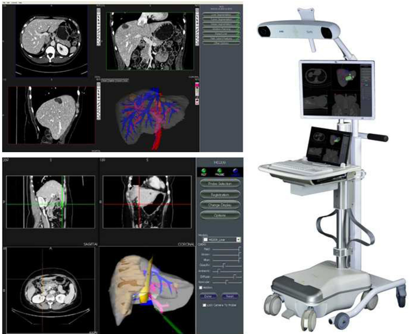
Figure 1. Screen captures of the software interfaces of the Scout™ Liver planning (top left) and Explorer™ Liver surgical navigation system (bottom left) are shown in addition to an image of the primary hardware associated with the Explorer™ Liver 3-D surgical navigation system (right panel).
