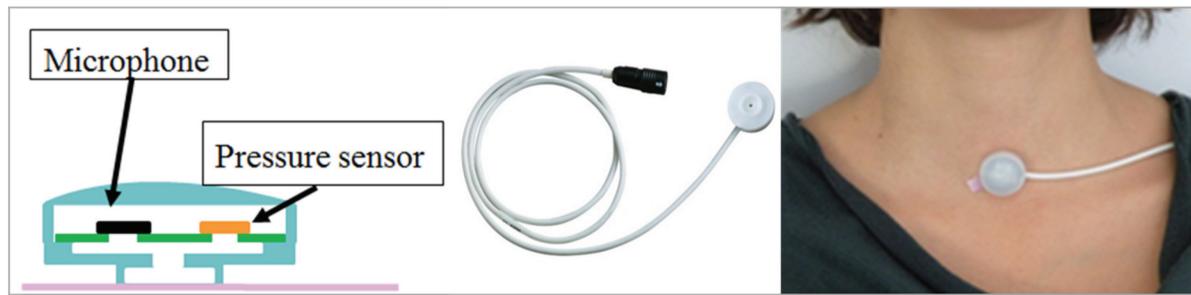
Figure 1 —Diagram of the PneaVoX transducer.
