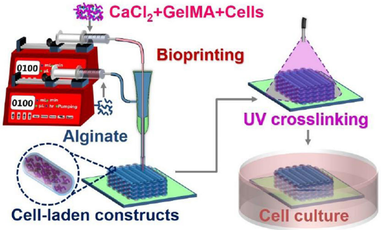
Figure 1. Schematic diagram showing the strategy of bioprinting GelMA/alginate core/sheath microfibers into 3D constructs with tunable microenvironments.
