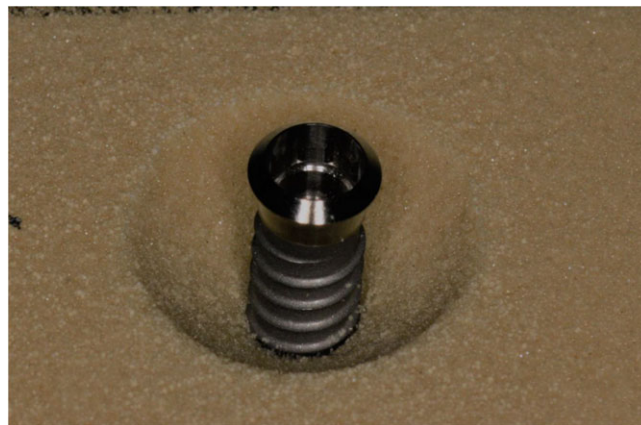
FIGURE 1 Experimental model showing the defect in Sawbone around the implant fixture
