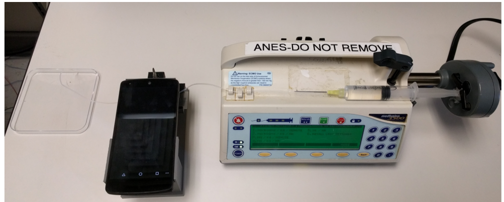
Fig 11. System setup to automate sample counting process using syringe pump, mobile phone on printed jig, and container to catch the samples after processing.
