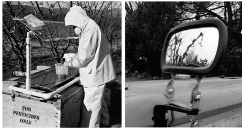
Figure 2. New and novel solutions found to be useful and acceptable after orchard field trials. (Left) Splash shield. This splash shield provides added eye protection for handlers when handling liquid pesticides. It also has a clipboard to hold the recipe and a metal tray to catch drips. (Right) Convex side view mirror. This mirror allows the handler to check on the spray pattern without turning his head all the time. It reduced his neck strain as well.
