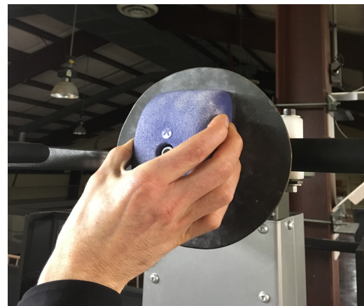
Figure 1b. A pinch grip being used on an indoor climbing hold. The climbing hold was attached to the training device, which was then assembled onto the WAPU.
