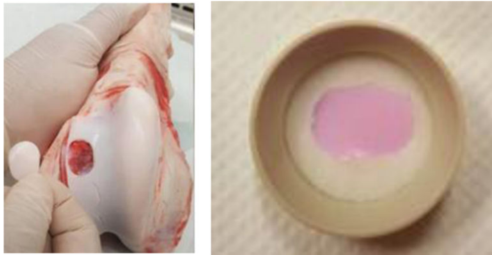
Figure 1. Cartilage procurement for friction testing. (a) Cartilage explant from the trochlear groove 20 mm in length and 14 mm in width (b) cartilage explant contained in porous polyethylene scaffold and stained pinkish after three days of pre-culture in culture medium.
