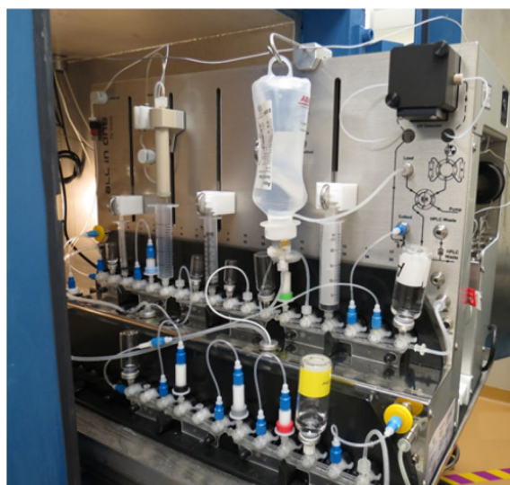
Fig. 2 AllinOne synthesis module with mounted disposable kits and reagents for [ ^{18}\text{F} ]F-Gln
