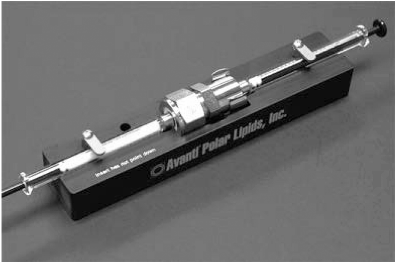
Figure 2. Fully assembled extruder apparatus (source www.avantilipids.com ; used with permission of Avanti Polar Lipids).
