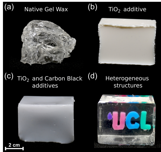
Fig. 1. Photographs of gel wax phantoms with different compositions. (a) Optically transparent native gel wax, prior to processing. (b) Native gel wax with \text{TiO}_2 added for optical scattering. (c) Native gel wax and \text{TiO}_2 , with carbon black ink added for optical absorption. (d) The University College London (UCL) logo fabricated with inclusions that comprised \text{TiO}_2 and differently-coloured inks in a native gel wax background ( Visualization 1 ).
