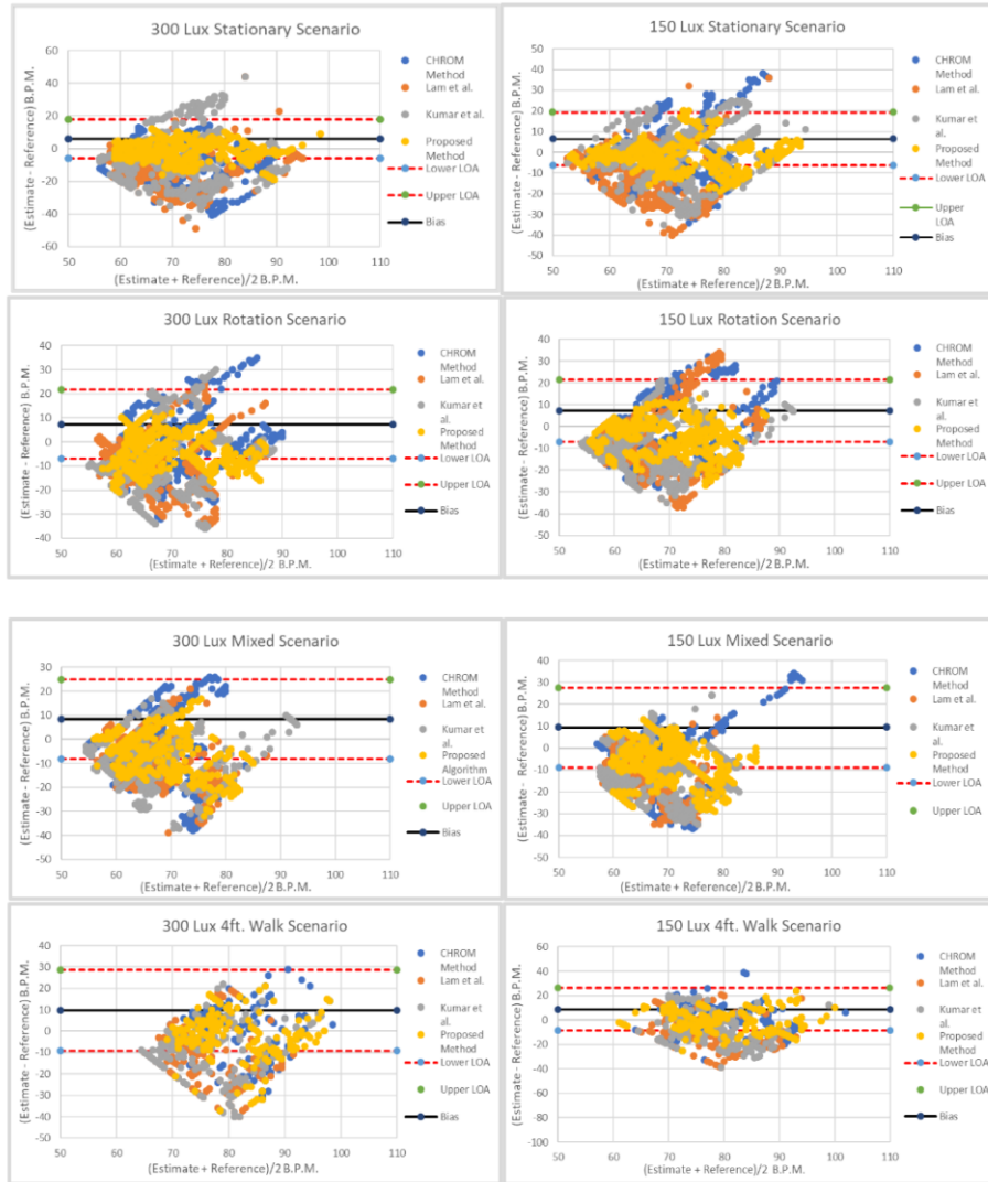
Fig. 13. Bland-Altman plots for four motion-scenarios in two illumination conditions. The Bland-Altman agreements are calculated between rPPG-signals and HR_{gr} values.
