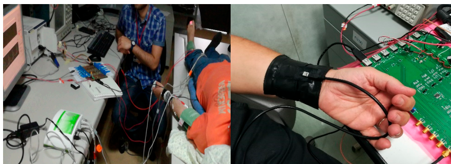
Figure 22. Some images of the validation setup used in our laboratories. In the first image we compare the processed PPG/ECG time-series with same ones obtained by commercial PPG/ECG medical device.
