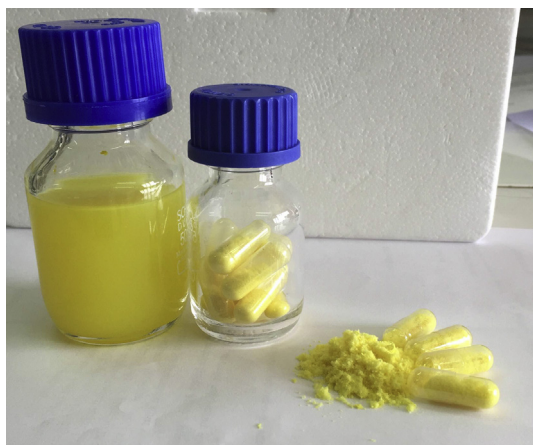
Fig. 13. The final curcumin and piperine loaded zein-chitosan nanoparticle product dispersed in a mixture of glycerole (19%, w/w) and water and as powder filled in capsules.
