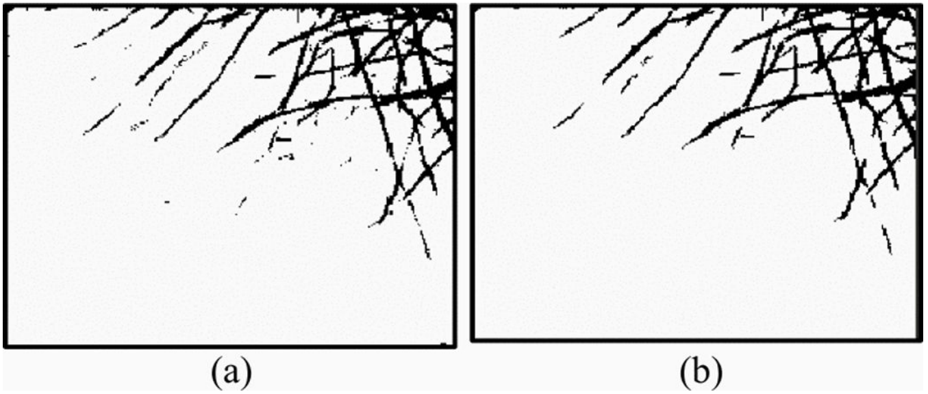
Fig. 3. (a) Binary image obtained by Otsu's threshold; (b) Noise removed
