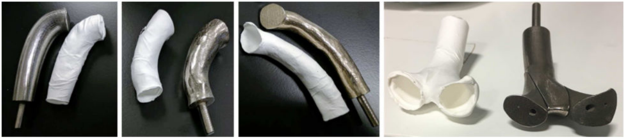
Figure 7. Pairs of 3D printed mandrels and electrospun biodegradable grafts (white). The pinned three-part design of the mandrel for bifurcated grafts can be seen on the right.
