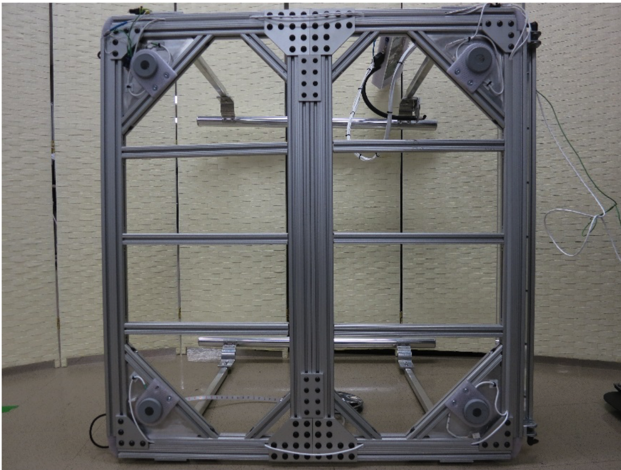
Figure 4. Bottom view of the adapted Wii Fit Balance Board braced for rigidity.
