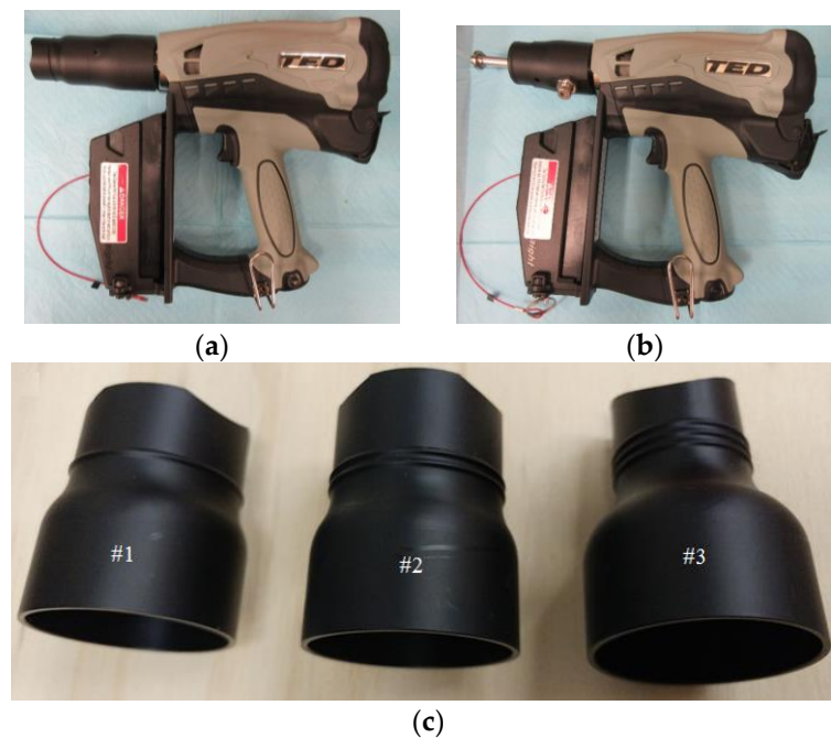
Figure 2. The non-penetrating captive bolt device (Turkey Euthanasia Device). (a) Device with adapter 1; (b) Device with adapter removed and bolt head exposed; (c) Subject adaptors [36].
