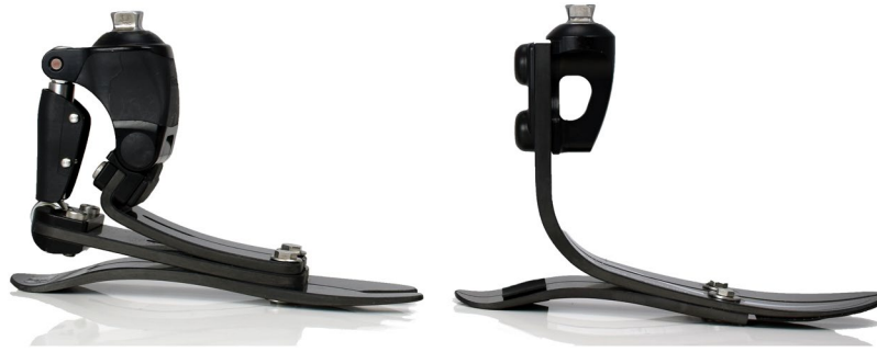
Figure 1. The Pro-Flex foot (left) has a linkage system on the upper portion of the foot that is designed to non-linearly load the heel and forefoot sections. This is a departure from conventional energy storage and return type prosthetic feet like the Vari-Flex (right).
