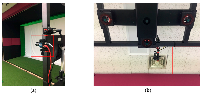
Figure 3. The cameras used for capturing images along with the wearable sensor: (a) the side view camera; and, (b) the top view camera.
