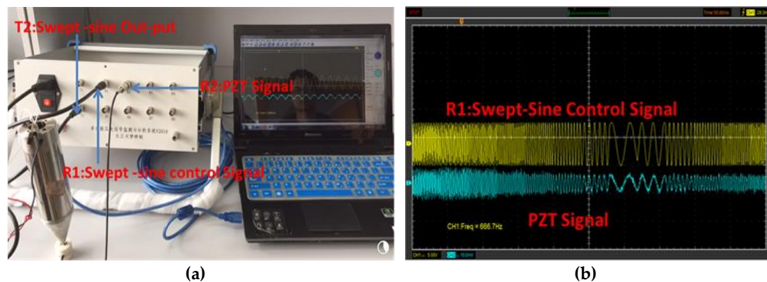
Figure 7. Sweep sine signal test. (a) Instrument setup for generating sweep signal; (b) Generated sweep signal waveform.
