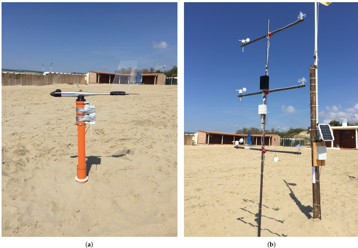
Figure 9. The nodes deployed on the Marina di Tirrenia beach, Pisa, Italy: (a) the sand trap and (b) the anemometer-anemoscope structure. The upper black box fixed in the middle of the anemometer-anemoscope structure houses the Coordinator. In the background it is possible to notice the 10 W solar cell powering the two nodes.
