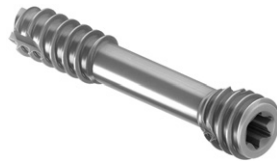
Fig. 1. The MAGNEZIX® CS resembles a cannulated conventional compression screw. It is made of a completely bioabsorbable magnesium alloy (MgYREZr).
