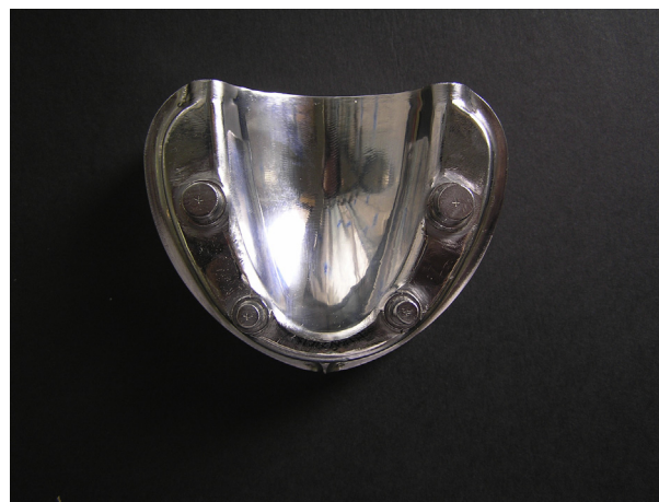
Fig. 1 CAD/CAM designed stainless steel die.
