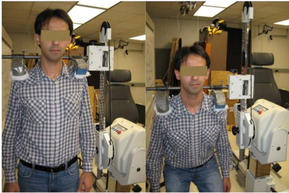
Figure 2. Customized Biodesign attachment for measurement of maximum voluntary exertions.
