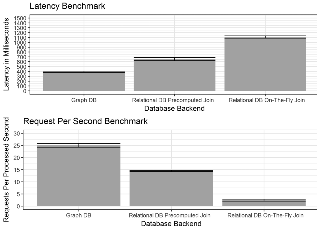
Figure 3. Metaviz database architecture benchmarks. We use the wrk tool to benchmark UI requests to three database architectures for storing abundance matrices and feature hierarchies (taxonomies): (i) Graph DB, using Neo4j with a Python Flask web service, (ii) Relational DB Pre-computed Join, using a MySQL implementation with a JOIN of the three tables of features, values and samples pre-computed and stored as a table, (iii) Relational DB On-The-Fly Join, a MySQL implementation with computing a JOIN across the three tables for each query. For (ii) and (iii), a PHP application issues queries to the database in response to requests from the UI. We deployed each implementation on an Amazon EC2 t2.small instance and the dataset used across all instances consisted of 62 samples, 973 features and 7 hierarchy levels. The upper panel shows query latency including standard error across 5 days of measurements. In addition to the latency of processing each request, we also measure the number of requests per second processed providing a measure of throughput in our application. In both performance measures, we see significant benefits of a Python-Neo4j deployment compared to a PHP-MySQL stack for Metaviz tasks.
