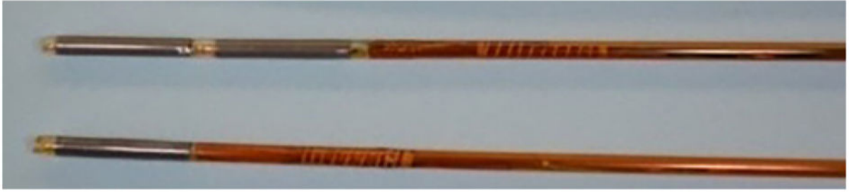
FIG. 2. Fabricated applicator with single ( bottom ) and double ( top ) transducer elements.
