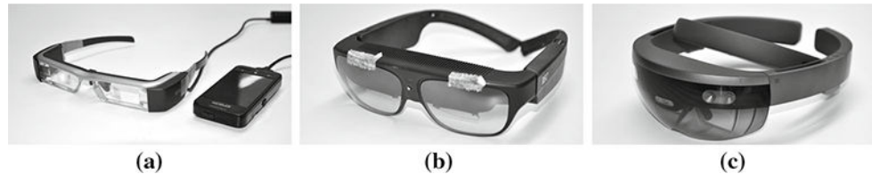
Fig. 3. Three optical see-through head-mounted displays for evaluation. a Epson Moverio BT-200. b ODG R-7. c Microsoft HoloLens
