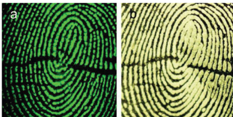
Figure 2. Latent fingerprint development on glass by using different types of developing powders: a) NaYF 4 :Yb, Er UCNMs, in dark field and under 980 nm NIR excitation; and (b) bronze flake, in bright field. Reproduced with permission. [73] Copyright 2014, Springer.
