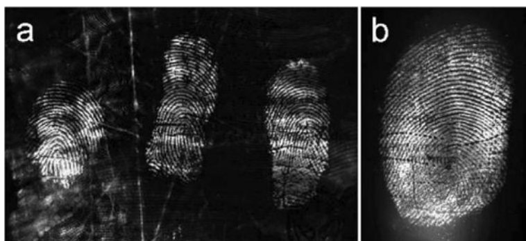
Figure 18. Latent fingerprint development on Australian five-dollar polymer banknote by using a) \text{NaYF}_4:\text{Yb,Er} UC powders and b) \text{YVO}_4:\text{Yb,Er} UC powders under the 980 nm NIR excitation. (a) Reproduced with permission [71] Copyright 2011, Elsevier. (b) Reproduced with permission. [72] Copyright 2012, Elsevier.
