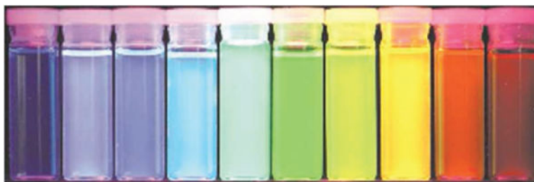
Figure 4. Aqueous suspensions of CdSe@ZnS QDs with ten distinguishable fluorescent emission colors excited with a 350 nm UV radiation. From left to right, the maximum emissions are located at 443, 473, 481, 500, 518, 543, 565, 587, 610, and 655 nm. Reproduced with permission. [47] Copyright 2001, Nature Publishing Group.
