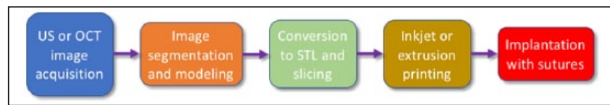
Figure 2. A concept map outlining the potential process involved in 3D printing an artificial cornea. Ultrasound (US) and optical coherence tomography (OCT) would be used to acquire the images upon which the model or artificial cornea is to be based; in cases of severely damaged or distorted corneas, US and OCT may primarily be of importance in gathering measurements relating to the surrounding structures. A 3D model is created from the acquired images through segmentation. The model is converted to standard tessellation language (STL) and sliced. Depending on which printing modality is chosen or developed for artificial corneal manufacturing, the model would be printed, likely through either an inkjet or extrusion-based system. The implant would then be placed by a qualified ocular surgeon in the same manner as a standard allograft.
