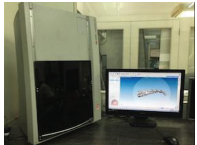
Figure 12: Photograph showing extraoral scanner (LAVA™ Scan ST Design system [3M ESPE]) and Dental Wings software
