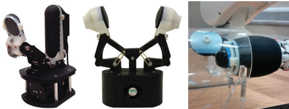
FIG. 2. The TacTip-M2 integrated into the open-hand model M2 gripper ( left ), the TacTip-GR2 mounted on the GR2 gripper ( middle ), and the TacCylinder in a simulated tumor detection experiment ( right ).
