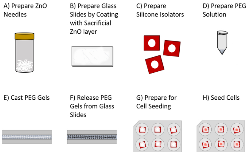
Figure 1. Schematic Overview of Hydrogel Preparation Protocol. A) Synthesis and collection of ZnO needles. B) Preparation of glass slides; creation of a sacrificial ZnO layer. C) Preparation and sterilization of silicone isolators. D) Preparation of PEG solution with ZnO needles. E) Polymerization of PEG gels between ZnO coated glass slides. White lines represent sacrificial ZnO needles and coatings. F) HCl rinse for the removal of needles and release of gel from slides. Dark lines represent pores created by dissolved ZnO needles. G) Transfer of gels and silicone isolators to 6-well dish to prepare for cell seeding. H) Cell seeding. Please click here to view a larger version of this figure.
