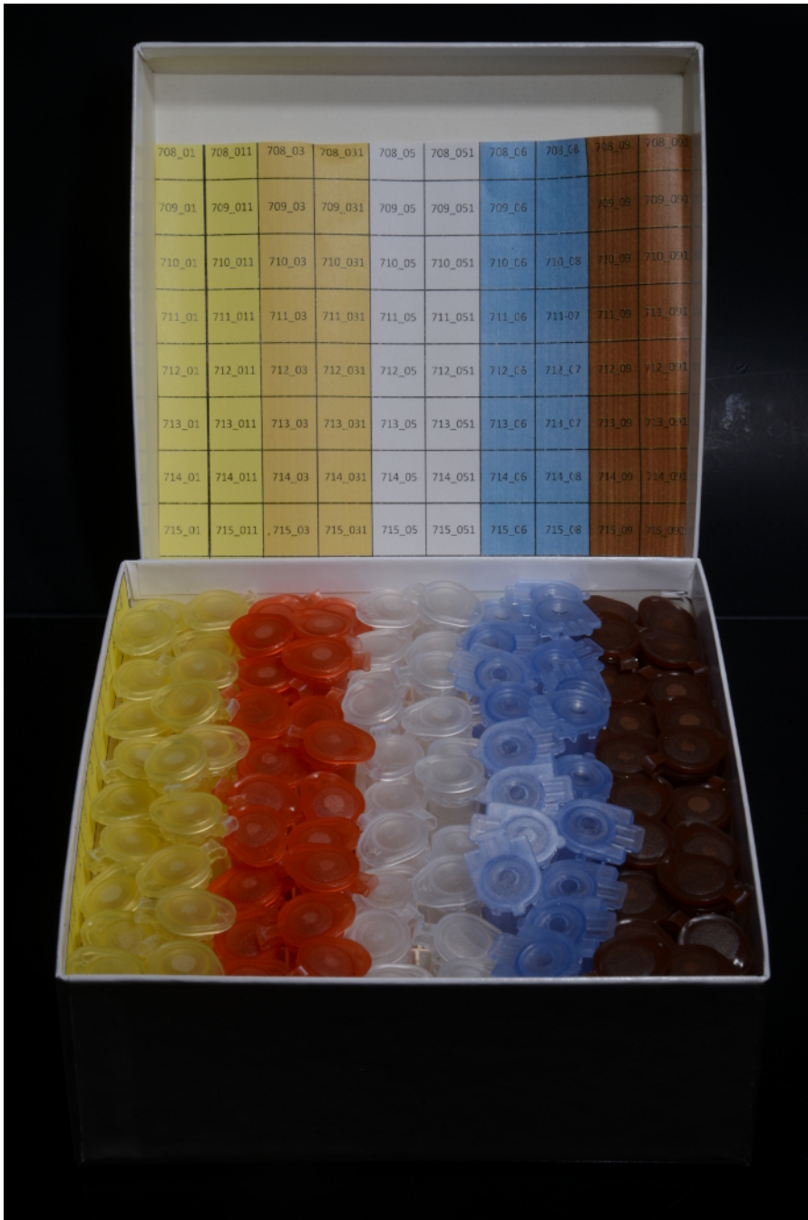
Figure 9: Color-coded storage. A referring color code for sheets and vials facilitates further sample handling. Please click here to view a larger version of this figure.
